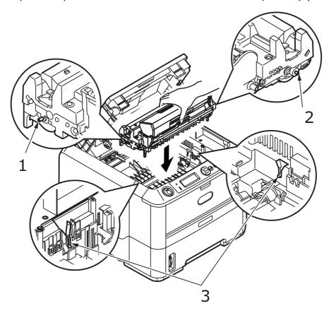
**6.** Lower the top cover but do not press down to latch it closed yet. This will protect the drum from excessive exposure to room lighting, while you check the remaining area for jammed sheets.
